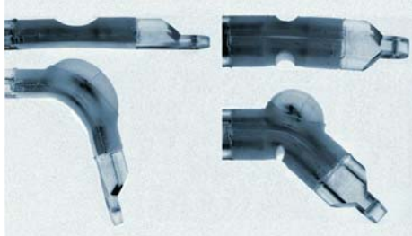
Monolithic manipulators could be realised with an adaptable gripping force and flexibility (ZENTNER, BÖHM)
